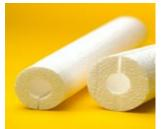
Thermotec SPI, foil faced, closed cell EPS polystyrene foam, has a nominal density of 13.5kg/m³. And is ideally suited to insulate chilled water lines in both industrial and commercial applications. Thermotec SPI Styrene can be supplied with a wall thickness that meets the effective R-value requirement of the BCA for chilled water services calculated to AS/NZS4859.1-2002
